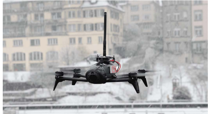
Fig. 1: Our prototype based on the COTS Parrot Bebop 2 quadrotor extended with our UWB-based localization unit.
